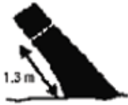
Figure (IX) DBH measurement position for an inclined tree.
