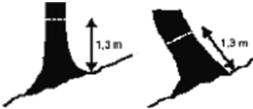
Figure (iv) DBH measurement position for a tree on steep terrain.
